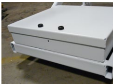
Hidden Ballast Compartment
